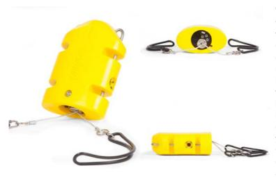
Would you shoot your gear without knowing when the trawl was starting to fill? Catch sensors have become key items of equipment, providing not just information on how fast the codend is filling up, but also giving vital indications on whether or not the gear is skewed, helping you avoid those lost tows. On top of all that, each catch sensor transmits a precise temperature reading to the wheelhouse.
