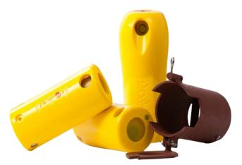
This lightweight trawl door sensor has been developed specifically for trawlers towing demersal trawls spread with a pair of pelagic doors flown off the seabed. This DS-70-W sensor is there to provide rapid, accurate information, allowing the skipper to be sure of the clearance between the door shoes and the seabed and to maintain a steady distance.
