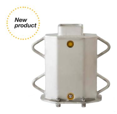
Fixed to a trawl's footrope, the Bottom Explorer provides a constant confirmation that the gear is in contact with the seabed, or an indication that the trawl has risen off the ground, giving the skipper the opportunity to respond by adjusting towing speed or warp length to place the gear back were it belongs. This minimises lost fishing opportunities and ensures that the trawl is actively on the ground.
