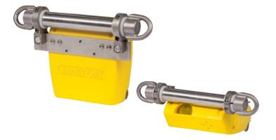
The Trawl Speed & Grid sensor is capable of measuring water flow in two axes, providing flow data as well as cross-current data, allowing corrections to be made to compensate for cross-currents when towing uphill or with mismatched warp lengths that can skew trawl geometry. Speeds of up to six knots can be monitored effectively and cross-currents of up to three knots are within the sensor's capabilities.
