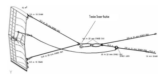
The range of measure will be **0 to 30 Tones** within an accuracy of **+/- 0.5%** and a repeatability of **+/0.25%** of Full Scale.
